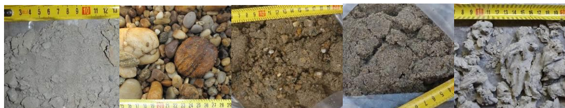
JDS14–Gabčíkovo r. JDS15–Medvedov JDS19– Iza/Szony JDS26 – Baja JDS45–Irongate r. Fig.30: Bed material samples – Middle Danube
