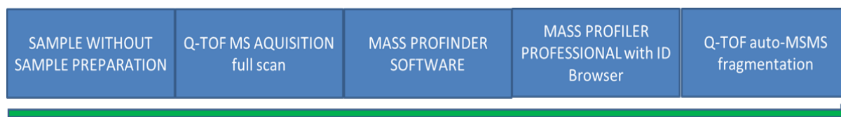
Figure 158: Non-target workflow used for analyses by UHPLC-Q-TOF-MS
